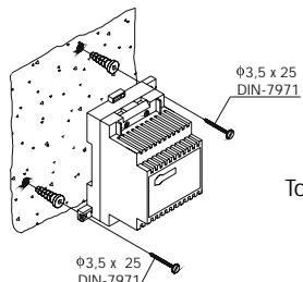
The power supply must be installed in a dry and protected place. It's recommended to protect the power supply by using a thermo-magnetic circuit breaker and to use a ground connection.
