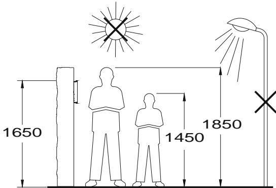
The upper part of the door panel should be placed at 1,65m.
