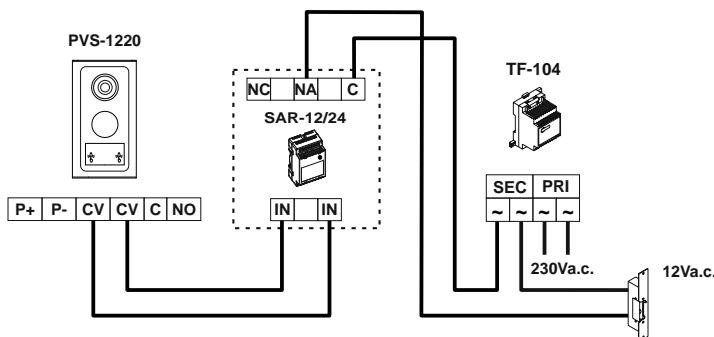
**C**onnection of an auxiliary device or control for gate automation.
