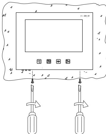
With help of a plain screwdriver, fix the monitor with specified screws, as shown on the picture.
