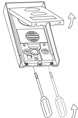
With help of a plain screwdriver, remove the aluminium front making a light pressure in the door panel bottom holes, as shown on the picture.
