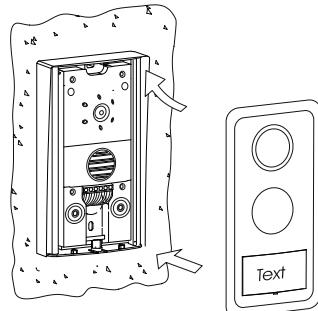
With help of a plain screwdriver, fix the aluminium front with especified screws, as shown on the picture.
