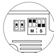
**IMPORTANT:** Modify the configuration switches without the power connected.
